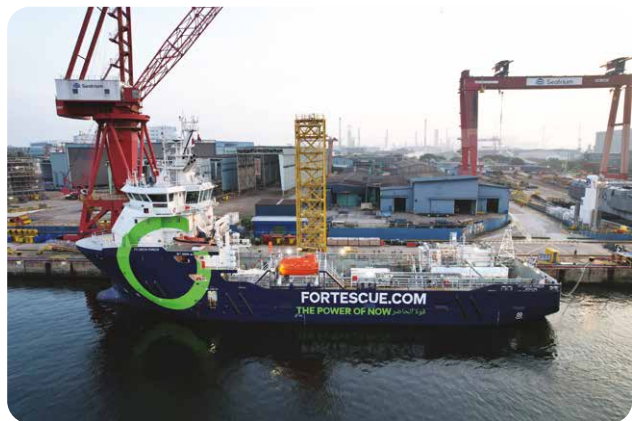
Successful conversion of FFI Green Pioneer, the world's first green ammonia-capable dual-fuelled vessel
