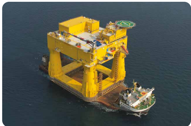
Sailaway of 900MW HVDC Offshore Converter Platform, DoWin epsilon, to Norway for the next phase of works following construction completion in Singapore
