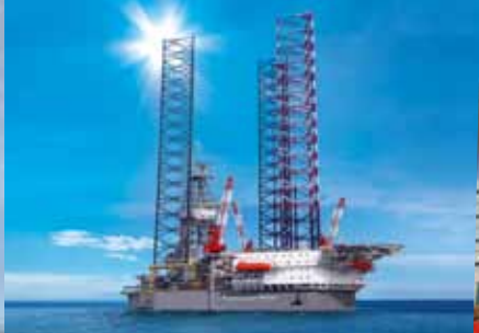
Transocean Honor , first proprietary Pacific Class 400 design jack-up rig
