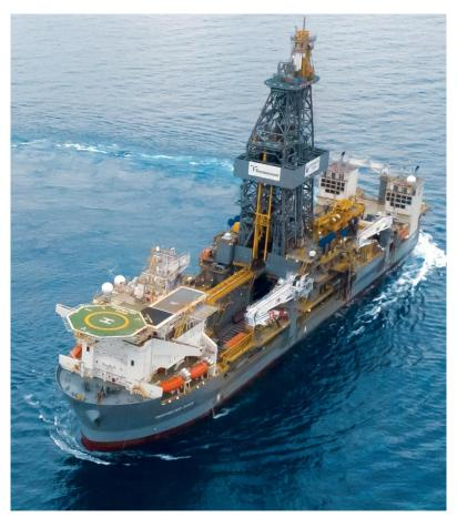
Deepwater Titan – the world's second 8th-generation drillship built for Transocean based on Sembcorp Marine's proprietary Jurong Espadon 3T design – is the first-ever unit delivered with two 20,000-psi blowout preventers, well-control, riser, and piping systems for high-pressure and high-temperature drilling and completion operations (*Photo: Transocean, all Rights reserved*)
