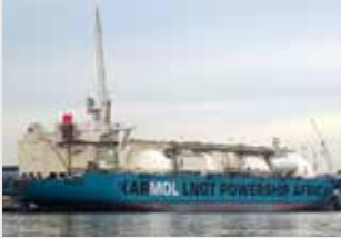
Conversion of Floating Storage Regasification Units from LNG tankers
